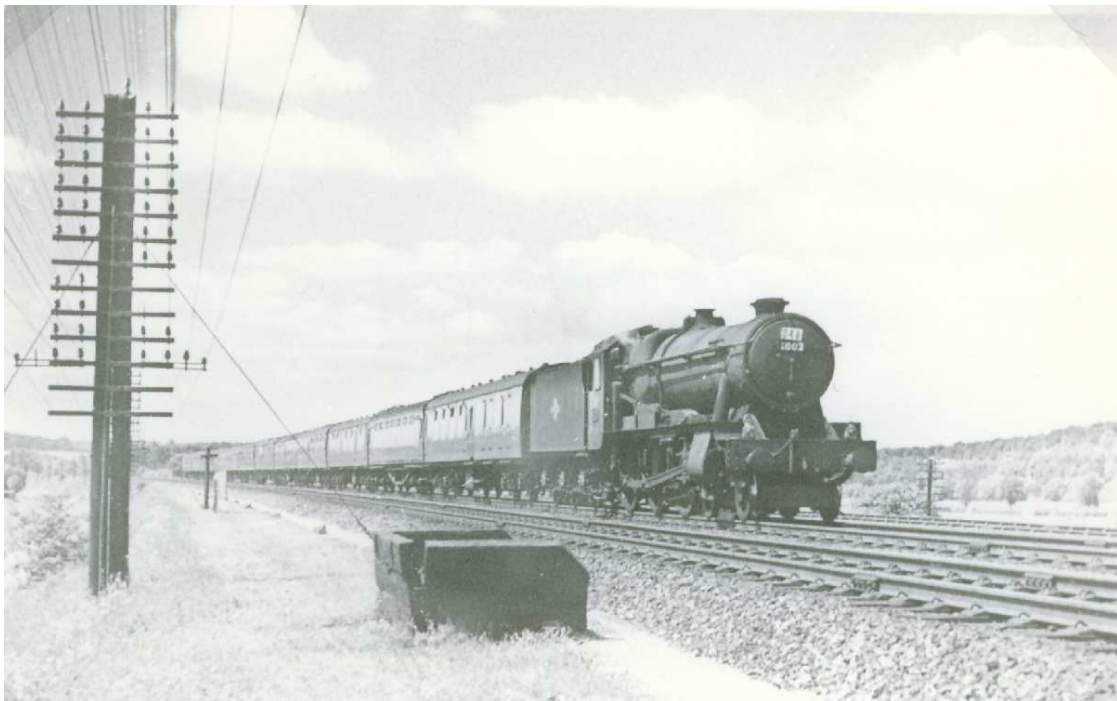
A County class 4-6-0 approaching Westbury Lane Bridge. These were rarely seen in this area./
